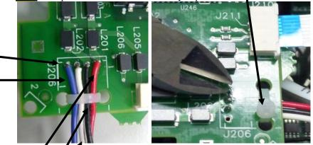
The **Red** wire is soldered in the main control board (reference E320) and should be soldered into pin #1 or the square pair of "J206" on the "A2" interface assembly.
