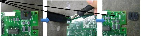
Remove the pins from the connector housing as shown. Cut 3cm off the clear tubing of the cable
