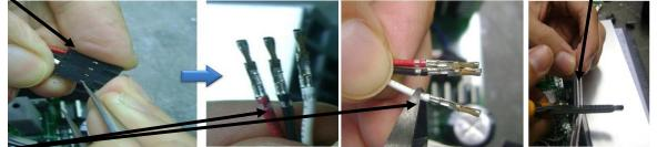
Cut the crimped terminals at the crimp around the wires colored insulation. This is done so the cable length can be as long as possible a short cable may cause assembly issues.
