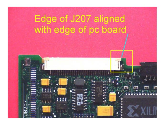
**CORRECT J207 PLACEMENT** – alignment to within < 0.3mm
