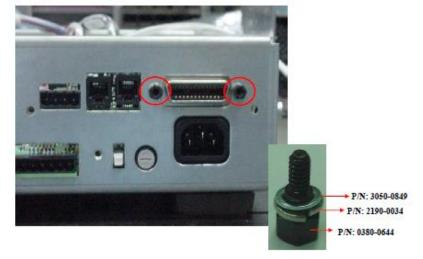
14. Secure with 2 screws as shown.
