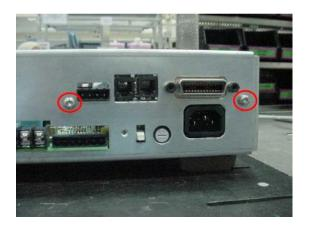
15. Connect long phone cable to J108 GPIB board as shown.
