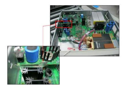
13. Use 2 flat washers, 2 split washers and 2 nuts and mount the GPIB board to rear panel.
