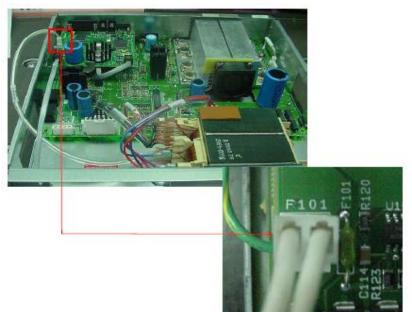
18. Insert the cable to J450 main PCA.
