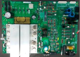
8. Place PCA into chassis on key slot 7 positions and push to lock in position at 7 locations. Use 5 screws to secure the board to chassis.
