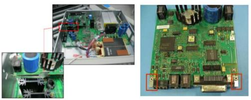
6. Remove 5 screws from the main board and slide out the PCA from the 7 slots, then remove the main PCA from chassis.
