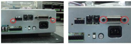
5. Remove bracket and GPIB PCA as shown.
