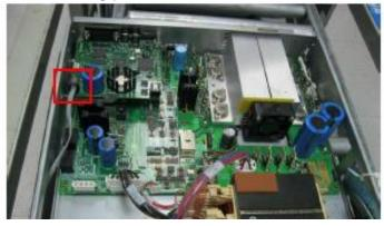
16. Connect short phone cable from J107 GPIB to J501 main PCA.
