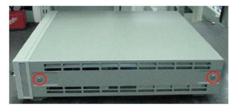
2. Slide cover out over chassis and remove the top cover. Then, remove the screw and ground cable.
