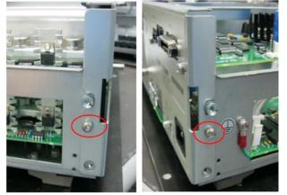
21. Attach cover block to the back cover and chassis by tighten the screw at each side.
