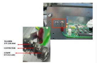
13. Tighten 2 screw as shown.
