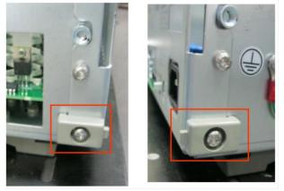
22. Mount the handle, front cap and back cap to both sides of cover with 2 screws as shown in the
