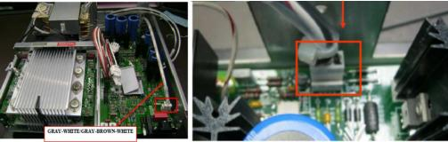
15. Connect cables from transformer, the number of cables varies base on model 6x51A, 6x52A, 6x53A, 6x54A and 6x55A.
