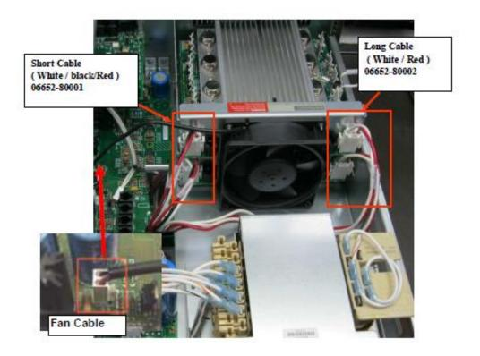
d. Disconnect 4 phone cables and cut the cable tie
