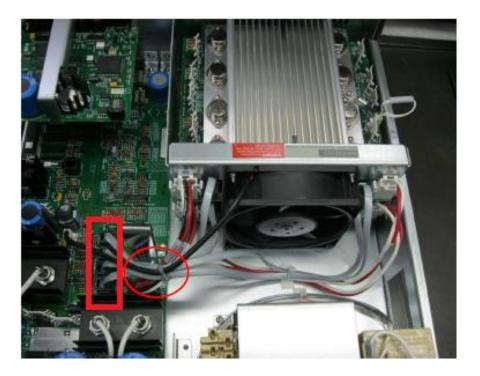
e. Disconnect cables from transformer, the number of cables varies base on model 6x51A, 6x52A, 6x53A, 6x54A and 6x55A.
