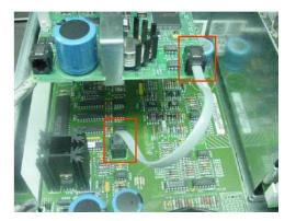
5. Disconnect white cable from transformer to the GPIB board as shown.
