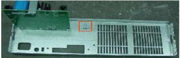
18. Connect phone cable from HPIB to the main PCA as shown.
