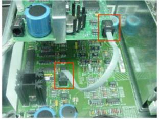
19. Connect white cable from transformer to the GPIB board as shown.
