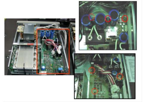
12. Tighten the ground screw.
