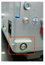
22. Mount the handle, front cap and back cap to both sides of cover with 2 screws as shown in the
