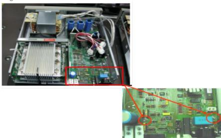
14. Insert cables J450 and J600 on PCA as shown.
