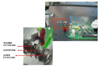
13. Tighten 2 screw as shown.
