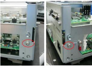
21. Attach cover block to the back cover and chassis by tighten the screw at each side.
