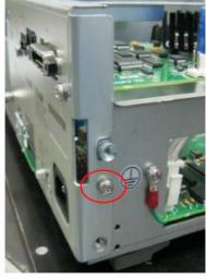
4. Disconnect phone cable from HPIB to the main PCA as shown.
