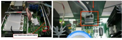
15. Connect cables from transformer, the number of cables varies base on model 6x51A, 6x52A, 6x53A, 6x54A and 6x55A.
