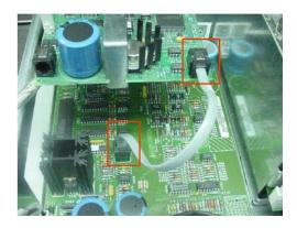
5. Disconnect white cable from transformer to the GPIB board as shown.
