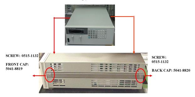
2. Remove cover block from the back cover and chassis after removed the screw at each side.
