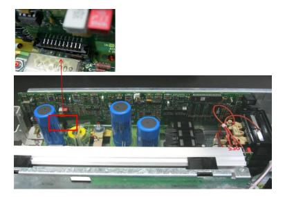
9. Insert standoffs of the control board into the holes of chassis and then, secure to chassis with 5 screws as shown in the following picture as below.
