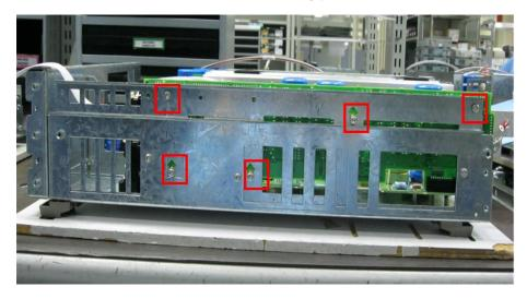
5. Slide out the affected board from the output board connector.
