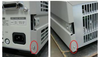
12. Mount the handle, front cap and back cap to both sides of cover with 2 screws as shown in the following picture as below.
