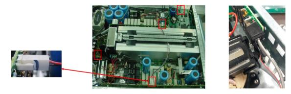
4. Remove 5 screws as shown in the following picture as below.
