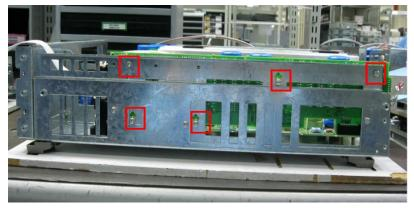
10. Connect and snap tight the phone cable and connector to control board with correct orientation as shown in the following picture as below.
