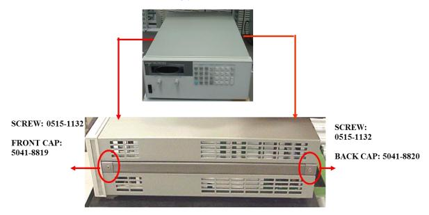
2. Slide cover out over the chassis and then, remove the top cover.
