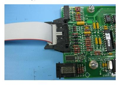
8. Place back the control board against the chassis and slide the board into output board connector. Then, slide the standoffs into the hole and push in place.
