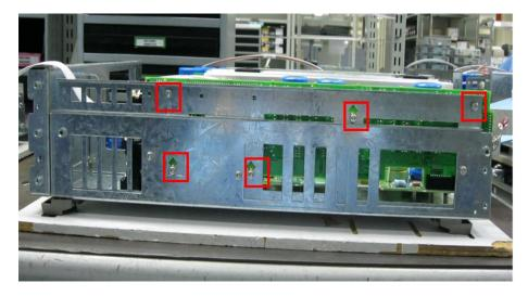
5. Slide out the affected board from the output board connector.
