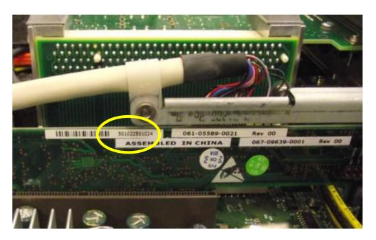
The board has a serial number (yellow circle)  ${\bf NOT}$  starting with 200... In the case above it is: 501022501024.
