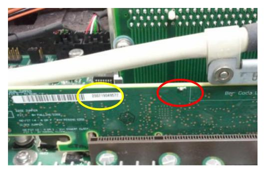
The board has a fuse on top (red circle) and a serial number (yellow circle) starting with 200... In the case above it is 200719049572)
