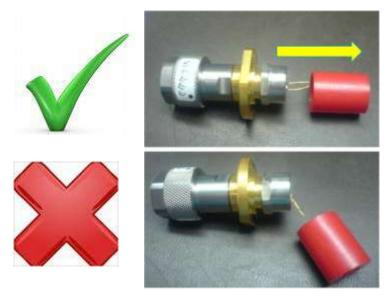
2 . If the wire is bent after removing the cap, use tweezers to straighten the bent wire as shown in the following figure
