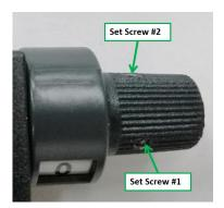
(4) After tightening both set screws, rotate knob counter-clockwise until it reaches the maximum attenuation (11/70/110dB). To ensure the attenuator functions properly, rotate the knob clockwise back to minimum attenuation (0dB), and repeat the movement for 10 cycles.
