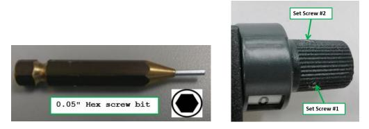
(4) After tightening both set screws, rotate knob counter-clockwise until it reaches the maximum attenuation (11/70/110dB). To ensure the attenuator functions properly, rotate the knob clockwise back to minimum attenuation (0dB), and repeat the movement for 10 cycles.
