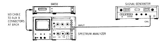
Figure 4-2. Insertion Loss Test Setup, Dc -1.8 GHz
