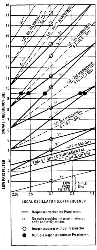
Figure 3-1. Spectrum Analyzer Tuning Curves and Responses
