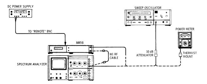
Figure 4-3. Insertion Loss Test Setup, 1.8 - 18 GHz
