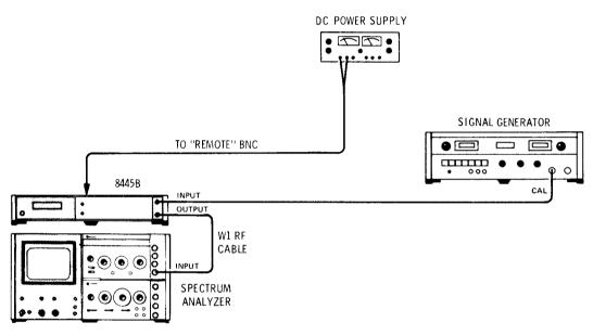
Figure 4-1. Out-of-Band Rejection Test Setup
