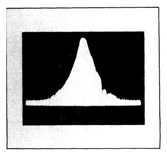
Figure 3-2. Typical 3-dB Yig Filter Pass band Display at 4 GHz and with a 10 MHz/DIV sweep.
