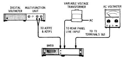
Figure 5-1. Power Supply Adjustment Test Setup
