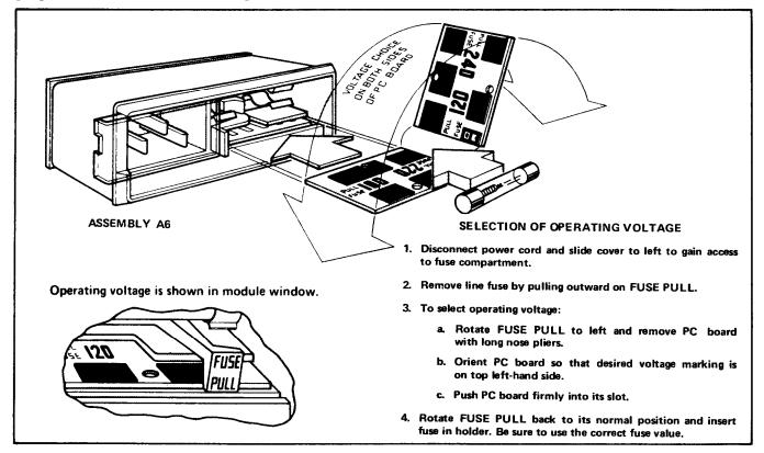
Figure 2-1. Line Voltage Selection
