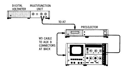
Figure 5-4. Digital Panel Meter Adjustment Test Setup.
