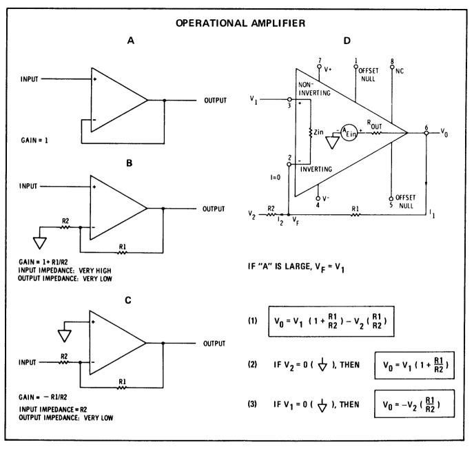
Figure 8-3. Operational Amplifier Equivalent Circuit
