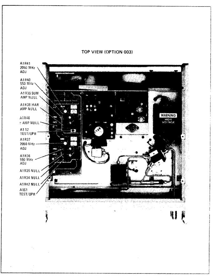
Figure 8-23. Option 003 A1 Adjustment Controls
