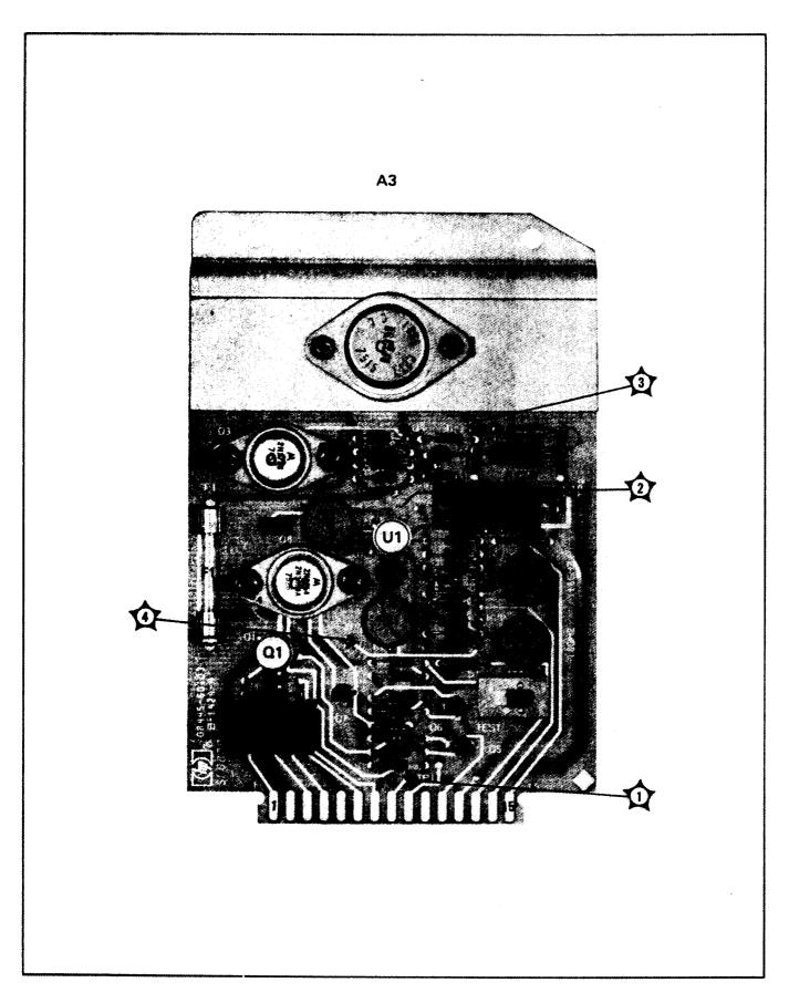
Figure 8-16A. A3 YIG Driver Assembly (Change 1)
