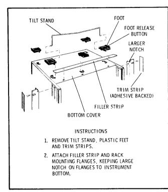
Figure 2-3. Preparation for Rack Mounting
