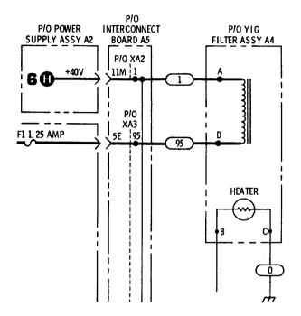
Figure 7-2. Partial Schematic correction for Service Sheet 4. (P/O CHANGE C)
