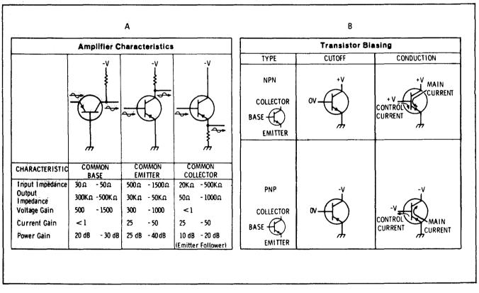
Figure 8-1. Transistor Characteristics and Biasing.
