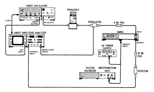
Figure 5-3. YIG Driver Adjustment Test Setup
