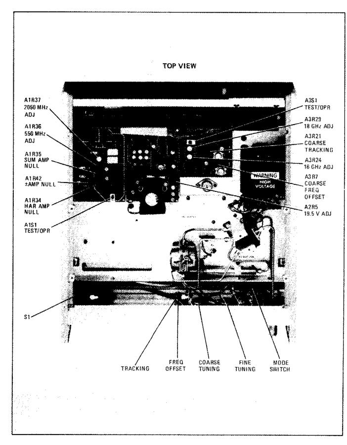
Figure 8-22. Adjustment Controls
