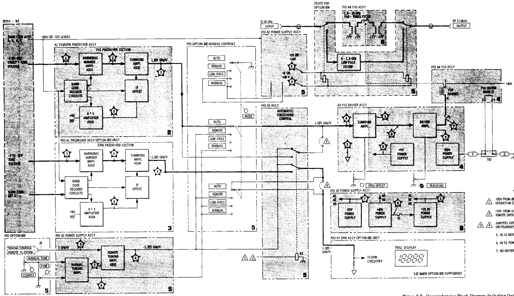
Figure 8-8. Comprehensive Block Diagram Including Options 002 and 003
