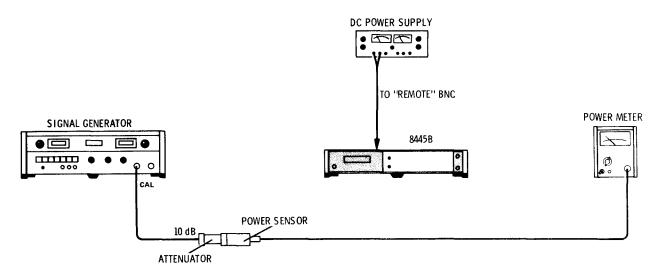
Figure 4-4. YIG Filter Signal Compression Test Setup
