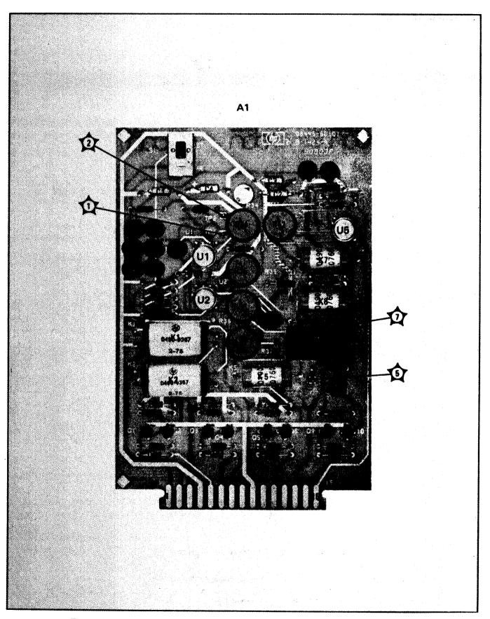
Figure 8-9A. A1 Predriver Assembly of 8445B (Except Option 003) (Change 1)
