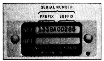
Figure 1-2. Serial Number Plate
