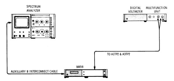
Figure 5-2. Pre-Driver Adjustment Test Setup
