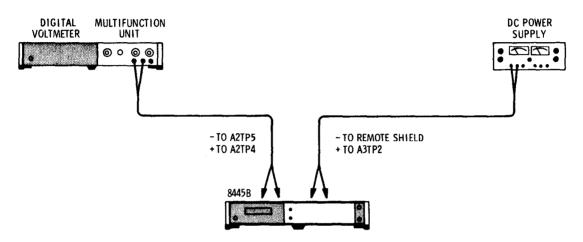
Figure 7-1. Remote Amplifier Adjustment Test Setup (Figure 5-3) (P/O CHANGE C)
