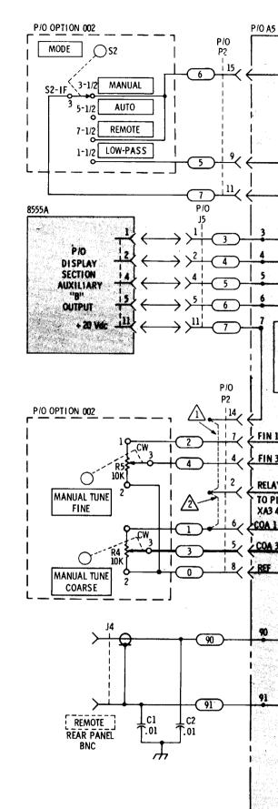
Figure 8-18. A2 Power Supply and Filter Switching Assembly
