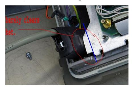
In the past some have attempted to increase the clearance by rotating the line switch 180 degrees, which may only result in a minor amount of additional clearance, and is not recommended.
