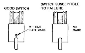
Figure 1. Pushbutton Front-Panel Switch, HP P/N 5060-9436
