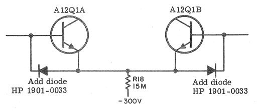
Figure 1. Schematic, Modified ALC Amplifier
