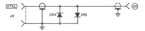
Figure 2. Schematic, Modified ALC XTAL Input
