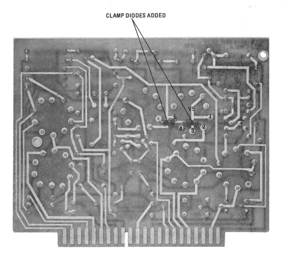
Figure 3. Modified A4 Helix Amplifier Board Assembly
