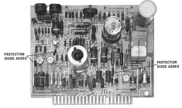
Figure 2. Modified A3 Reciprocal Amplifier Board Assembly
