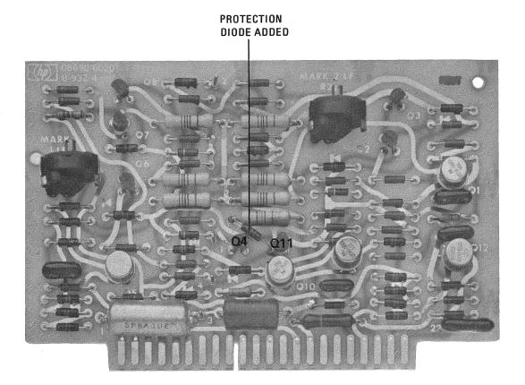
Figure 1. Modified A11 Amplitude Modulator Board Assembly
