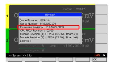
Step 2: If the firmware revision displayed is 2.2.1744.8725 or earlier, install the firmware 2.2.1831.4380 or later, following the procedure below.
