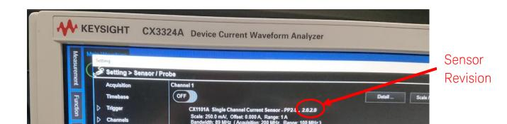
NOTE: If not displayed, click on "Channel 1" in the "Sensor/Probe" section to get the below. This explains the case when CX1101A is connected to Channel 1 port.
