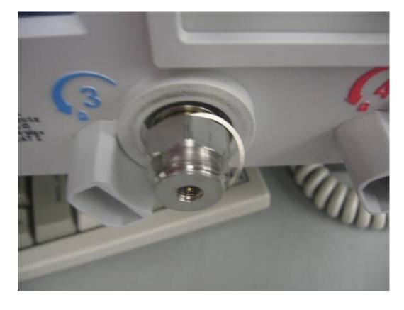
4. Slip the spring behind the bulk head connector as illustrated below.
