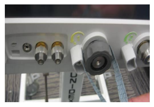
3. Slowly pull the strap or string to remove the clutch from the front panel.
