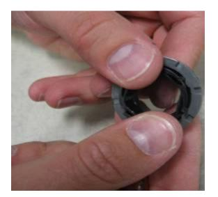
6. Press the assembled clutch onto the front panel.
