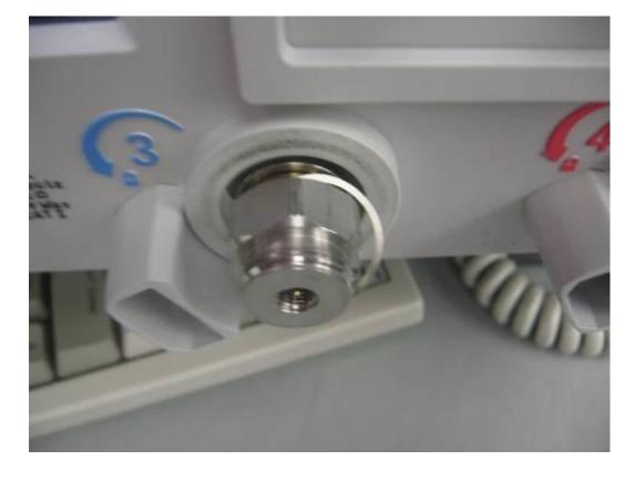
4. Slip the spring behind the bulk head connector as illustrated below.
