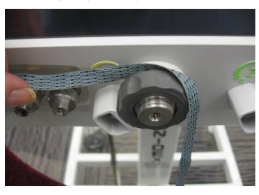
2. Put the soft strap or string behind the gray outer clutch and carefully work it around the outer clutch.
