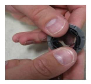
6. Press the assembled clutch onto the front panel.
