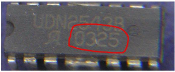
**Solution/Action:** A E1465A that fails to close or open it's relays and has the 0325 date code ICs should be replaced with a E1466-66701.
