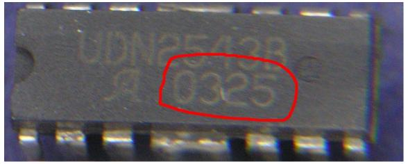
**Solution/Action:** A E1466A that fails to close or open it's relays and has the 0325 date code ICs should be replaced with a E1466-66701.
