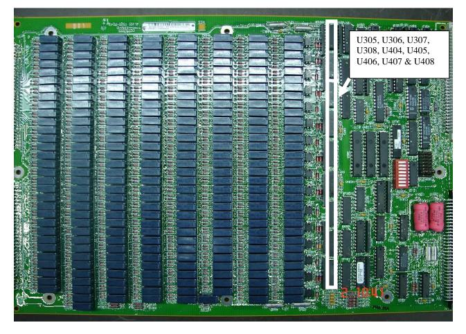
Part Number Location Impacted Reject Criteria : E1466-66501 : U305, U306, U307, U308, U404, U405, U406, U407 & U408 : DC 0325 on IC
