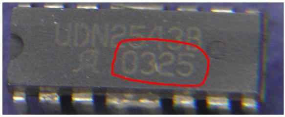
**Solution/Action:** A E1467A that fails to close or open it's relays and has the 0325 date code ICs should be replaced with a E1466-66701.
