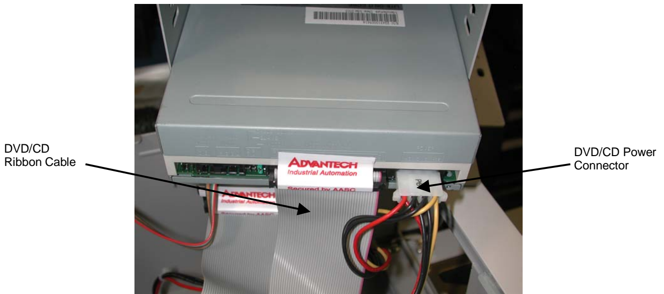
Figure 4. Removing the DVD/CD Ribbon Cable and Power Connector
