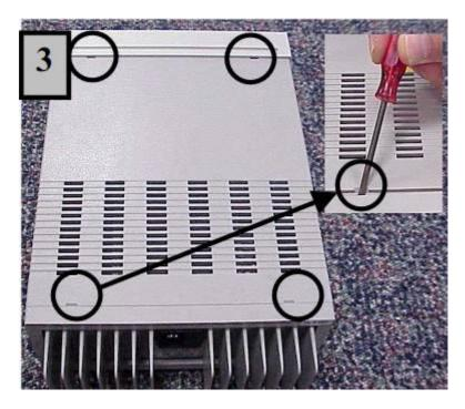
**REMOVE COVER** by prying rear bezel and front panel away from cover in four places as shown. Then lift cover off unit.
