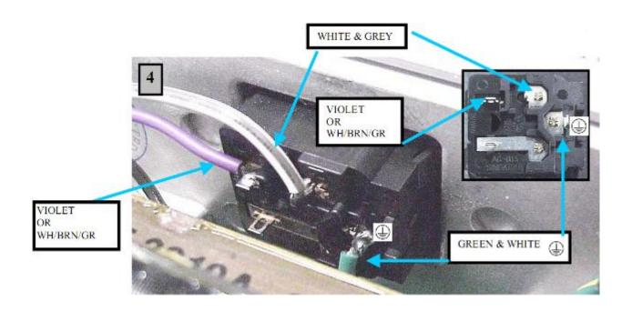
**REPLACE MODULE** with P/N 5065-6978. Before soldering perform "TEST FOR LOOSE AC MODULE" as shown in the picture above. This will confirm that the new module is secure. Solder wires and **REPLACE FUSE**.
