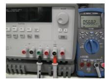
±25V output power line's common terminal to ground terminal
