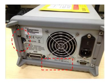
Figure 1: Loose rear bumper – gap observed between bumper and chassis
