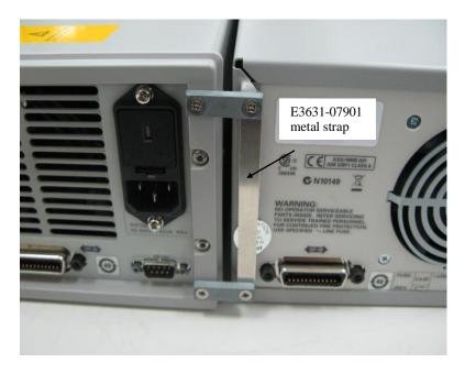
Figure 5: Rear view rear lock link secured with metal straps kit for side-by-side rack mounting
