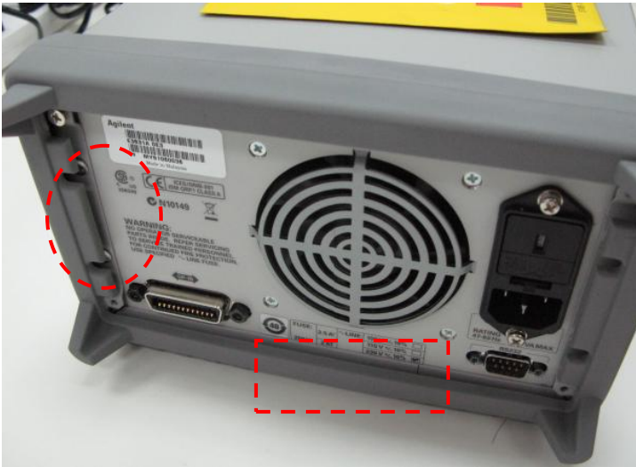
Figure 1: Loose rear bumper – gap observed between bumper and chassis
