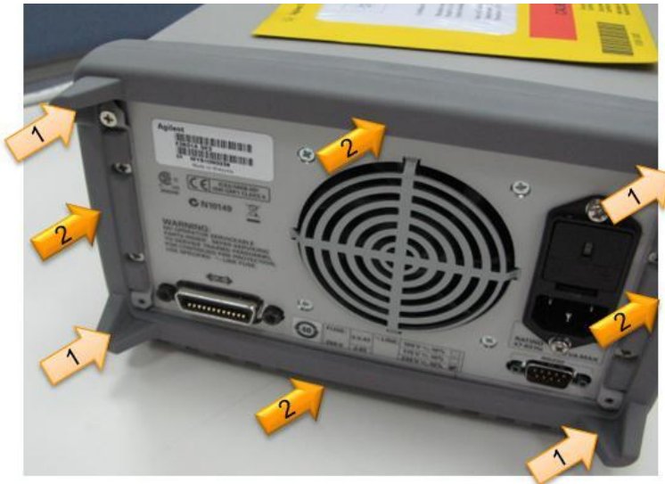
Figure 2: Proper fitting method for instrument rear bumper
