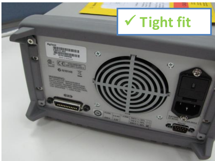
Figure 3: Tightly fitted rear bumper – no gap observed between the bumper and chassis
