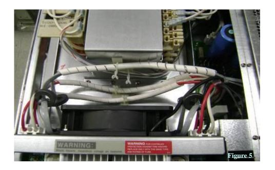
1) Secure the cable with cable clip (P/N1400-1281) as shown in figure 5.
