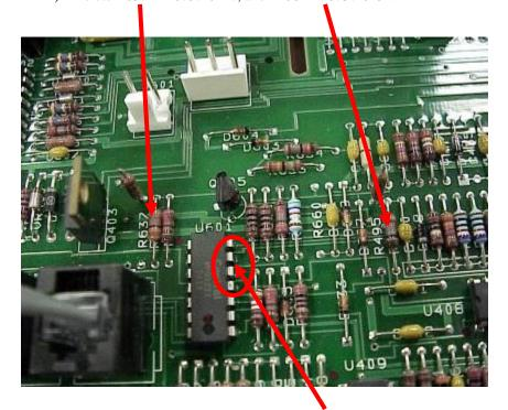
2) Add a jumper wire to connect U601 pins 12 & 13 together, on the bottom side of the PCB. Use a 26 AWG wire PN 8150-2408 19.75 mm long and strip 4 mm off each end.
