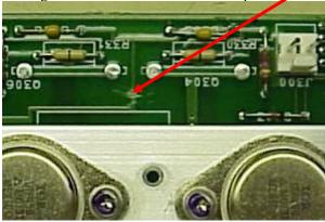
8. Add ground wire 22 AWG by wrapping and soldering wire from minus side of Solder to pin one of J300 Capacitor  $C_3^2$ 05.
