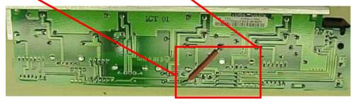
3. Add ground wire 22 AWG by wrapping and soldering wire from minus side of Capacitor C305 to pin one of J300.
