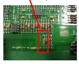
Note: Secure the added wire to PCB with epoxy or hot melt glue.
