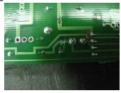
6. Cut ground tract from minus side of Capacitor C305 to minus side of source resistor R306.
