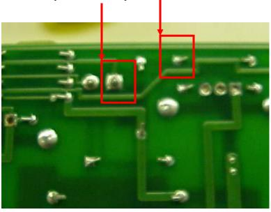
9. PCA with wire added modification for right tunnel assembly PN 5063-4815 for PCB 5020-2901 REV B completed.
