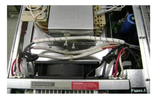
1) Secure the cable with cable clip (P/N1400-1281) as shown in figure 5.
