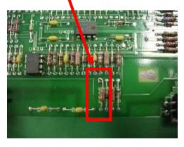
Note: Secure the added wire to PCB with epoxy or hot melt glue.
