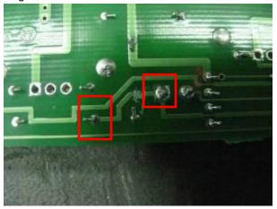
6. Cut ground tract from minus side of Capacitor C305 to minus side of source resistor R306.
