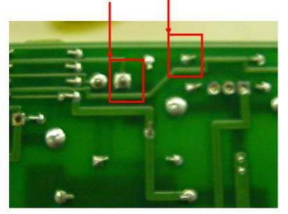
9. PCA with wire added modification for right tunnel assembly PN 5063-4815 for PCB 5020-2901 REV B completed.
