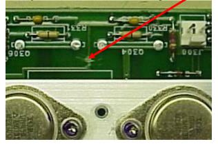
8. Add ground wire 22 AWG by wrapping and soldering wire from minus side of Solder to pin one of J300 Capacitor C305.
