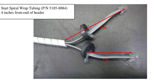
Place phone cable through core 3 inches from end of header and tie rap exactly as shown
