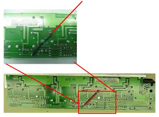
3. Add ground wire 22 AWG by wrapping and soldering wire from minus side of Capacitor C305 to pin one of J300.
