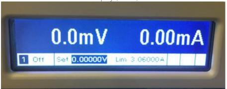
LCD (blue/white display assembly, part no. 2090-1031) has been discontinued by vendor. Replacement assembly (pictured later) is part no. 5067-5993 (amber in color). Difference in color doesn't impact any performance and specification. Unfortunately, this cannot be altered.
