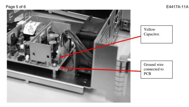
10) This picture above shows the ground wire connection to the PCB. Please be aware that the ground connection is very close to the leg of the yellow capacitor. PLEASE DO NOT LET THE GROUND WIRE TOUCHES THE CAPASITOR'S LEG.
