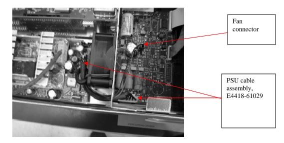
4) Replace with new PSU cable assembly E4418-61029. You can differentiate the cable assembly by the colors. The old cable is Black and new cable is RED.
