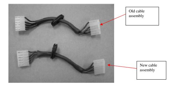
Note: If the power cable assembly is red in color, indicates that the cable already been changed. No action is needed.
