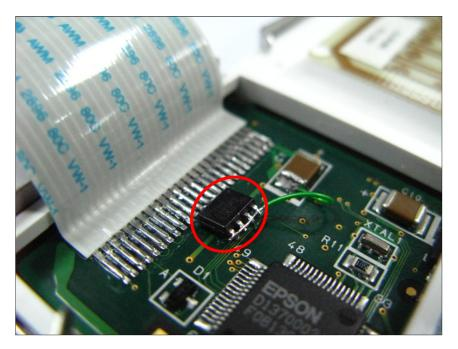
Front panel with older version of LCD display controller can also be used to resolve this problem. For more information on old and new version of LCD display controller, please refer to service note E4417A-13A.
