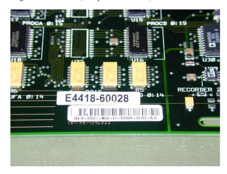
Figure 4. Application of New Label E4418-80025 to Component Side
