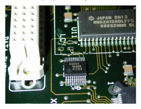
Figure 3. Surface Mount Resistors Removed from Board
