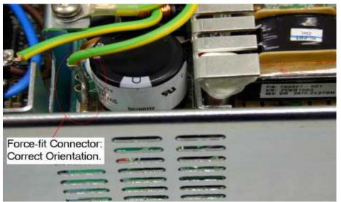
Figure 3: Correct orientation of force-fit connector.
