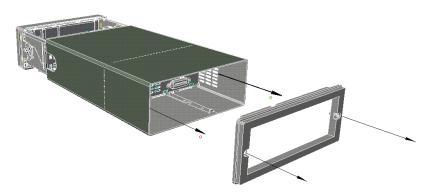
2. Remove the power supply cover by lifting it out as shown below.
