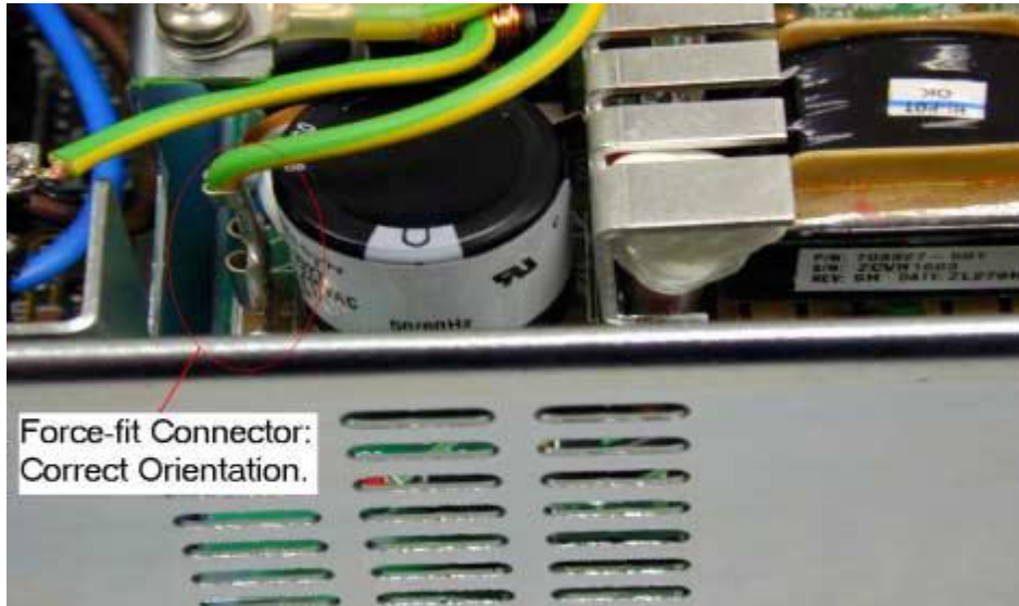
Figure 3: Correct orientation of force-fit connector.
