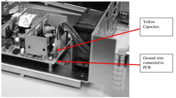
10) This picture above shows the ground wire connection to the PCB. Please be aware that the ground connection is very close to the leg of the yellow capacitor. PLEASE DO NOT LET THE GROUND WIRE TOUCHES THE CAPASITOR'S LEG.
