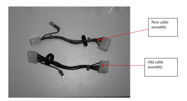
Note: If the power cable assembly is red in color, indicates that the cable already been changed. No action is needed.
