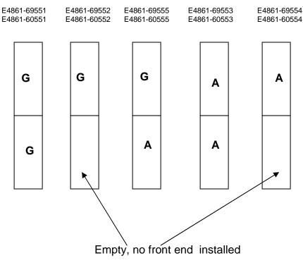
**G**: E4862B Generator installed in E4861B **A**: E4863B Analyzer installed ind E4861B
