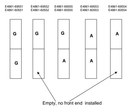
**G**: E4862B Generator installed in E4861B **A**: E4863B Analyzer installed ind E4861B
