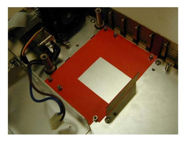
Step3. Place the power supply on the insulator. After fastening the power supply, remove the film of adhesive tape of the insulator. Then, fasten ANGLE SHIELD (E4980-01205) and stick the adhesive part of the insulator to the ANGLE SHIELD
