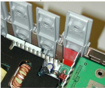
Step5. Check whether the insulator is placed correctly. Look at the inside through the hole of the right-side wall of the chassis with a flashlight. You can find the red color tab.
