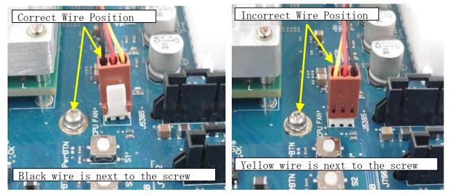
2-2. If black wire of the CPU fan cable is next to the nearby screw, J19 is assembled in a correct way.
