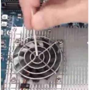
2. If CPU fan rotates, then the cause of the trouble is [dropped off rotor]
