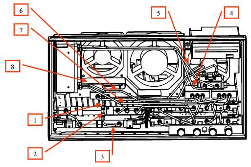
Figure 14 Front View (Semirigid Cables Opt. 413, 414 after modification)
