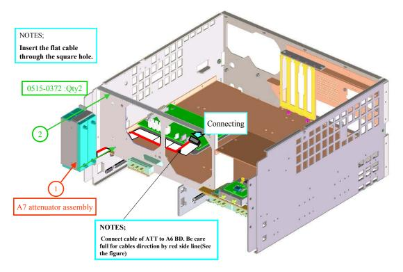
Figure 9 Install A7 attenuator assembly (for option 313, 314, 413, 414)
