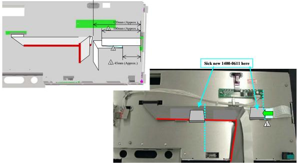
New cable cramp position and cable bending reference
