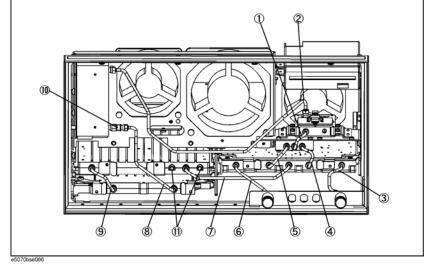
Figure 6 Front View (Semirigid Cables Opt. 214 before modification)
