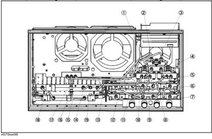
Figure 13 Front View (Semirigid Cables Opt. 413 before modification)
