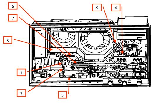
Figure 10 Front View (Semirigid Cables Opt. 313, 314 after modification)
